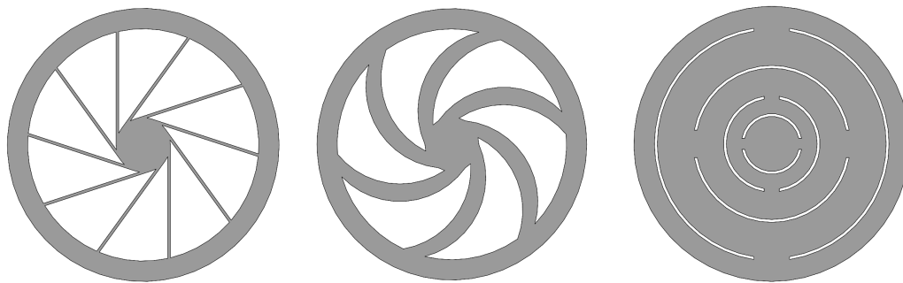
Figure 8. Diaphragm design using (left) wire flexures, (middle) curved blade flexures, and (right) slits.
