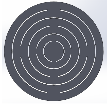
Figure 24. Modified series slit diaphragm design after topology optimization study.
